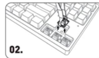
02. Use a switch puller to pull out the switch body
