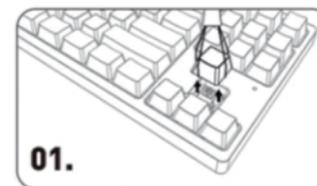
01. Remove the key cap with a key puller
