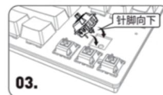
03. Check the installation position of the switch
